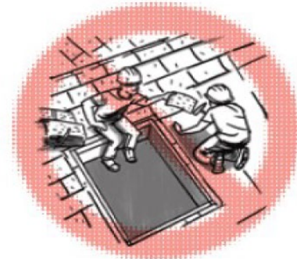
DON'T work around unprotected openings or skylights
