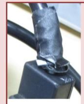
Do not use damaged or cracked power cords. Do not try to repair them with electrical tape! Inspect cords regularly for damage.
