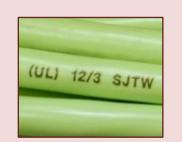
**Grounding:** Extension cords must be 3-wire type so they may be grounded, and to permit grounding of any tools or equipment connected to them.
