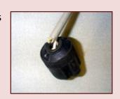
Cord Damage: A flexible cord may be damaged by door or window edges, by staples and fastenings, by abrasion from adjacent materials, or simply by aging. If the electrical conductors become exposed, there is a danger of shocks, burns, or fire.
