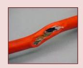
Durability: The OSHA construction standard requires flexible cords to be rated for hard (300V) or extra-hard (600V) usage. These ratings are derived from the National Electrical Code and are required to be indelibly marked approximately every foot along the length of the cord. Examples of these codes are; S, ST, SO, and STO for hard service, and SJ, SJO, SJT, and SJTO for junior hard service.
