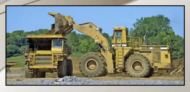
Operators and bystanders should remember: the danger zone of heavy equipment includes the area reached by any attachment and by the load.
