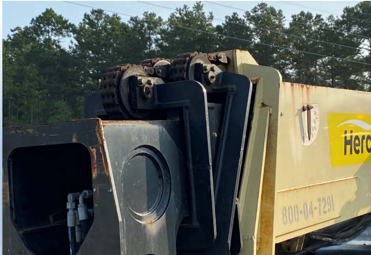
Inadequate lubrication on the tracks.
