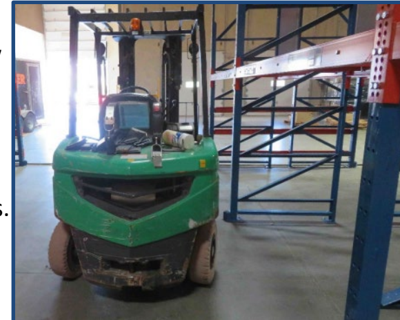
Rear side of forklift that struck and crushed the operator against one of the metal uprights.
