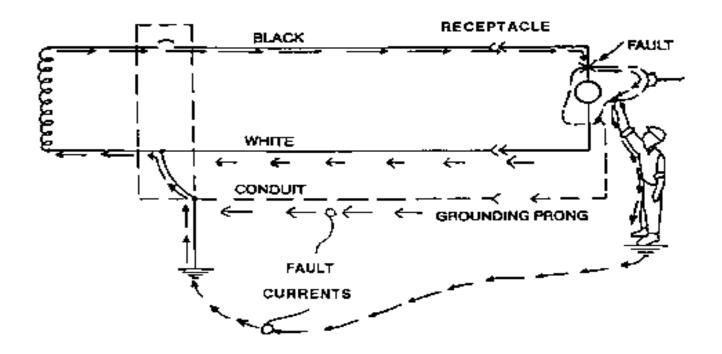
Figure 15: FAULT CONDITIONS SENSED BY A GFCI
