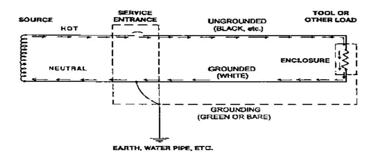
Figure 12: CURRENT FLOW IN A PROPERLY GROUNDED CIRCUIT
