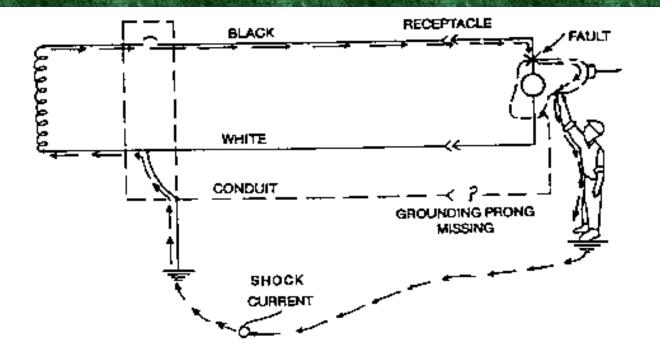
Figure 14: SHOCK FROM IMPROPERLY GROUNDED TOOL
