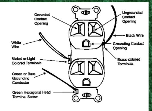
Figure 16: CORRECTLY WIRED DUPLEX RECEPTACLE
