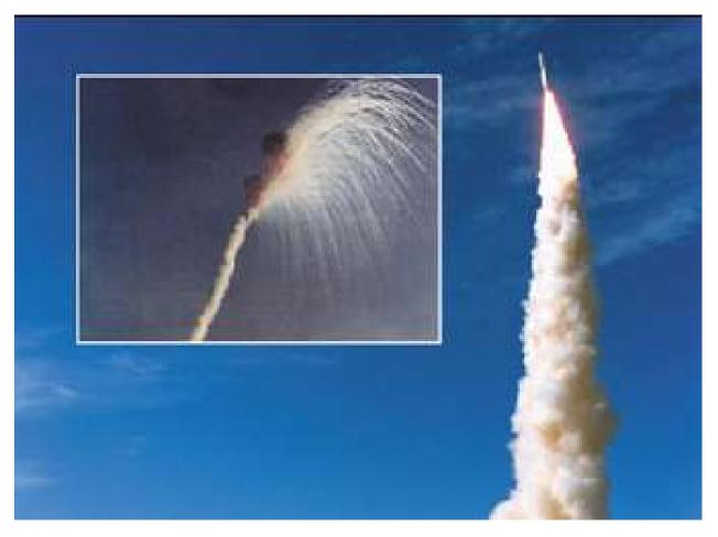
The explosion of a Titan IVA with a NRO satellite in August 1999 was caused by wiring defects. Titan IV quality defects were linked to the overemphasis on cost cutting and the loss of experienced personnel.
