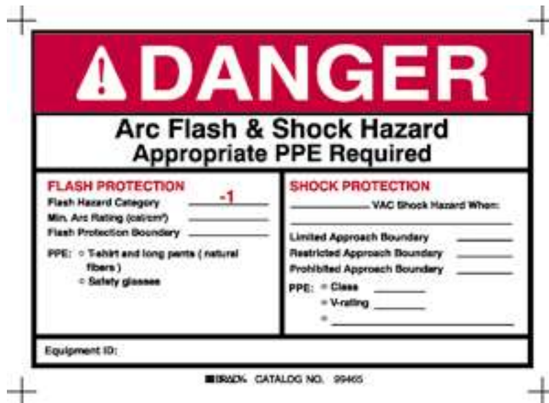
Figure 2. Post-analysis Arc Flash Hazard Label.
