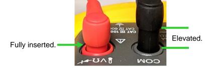
D. Securely short the clean probe tips of the test leads together to maintain continuity throughout the test. **They must maintain contact throughout this test.**
