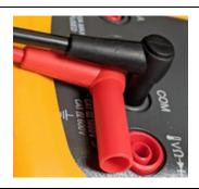
C. While leaving the black test lead elevated, fully insert the red test lead.
